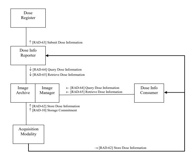
Figure 22.1-1: Radiation Exposure Monitoring - Actor Diagram
