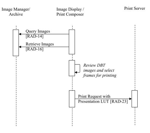
Figure 37.4.2.6.2-1: Process Flow in Printing of Selected DBT Frames Use Case
