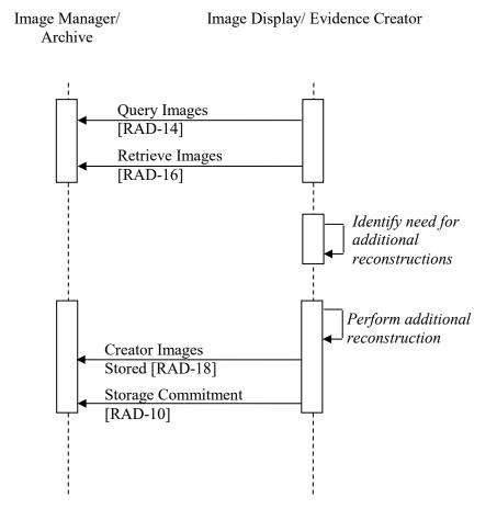
Figure 37.4.2.2.1: Process Flow in Additional Reconstructions Use Case
