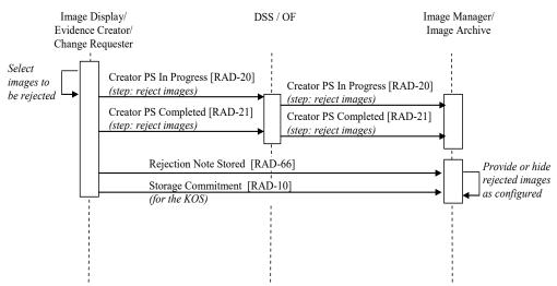
Figure 28.4.2-1: Process Flow for handling rejected images
