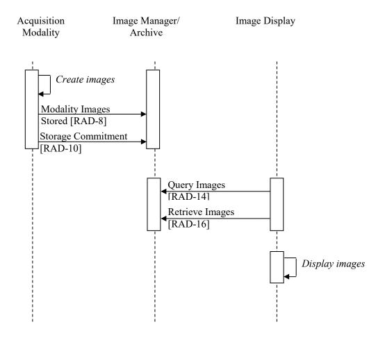
Figure 37.4.2.1.2-1: Process Flow in DBT Screening Use Case
