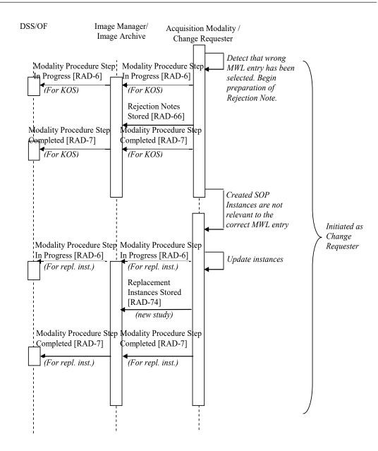
Figure 28.4.4-3: Acquired Images are Not Relevant to Correct Procedure and are Handled as an Unscheduled Case
