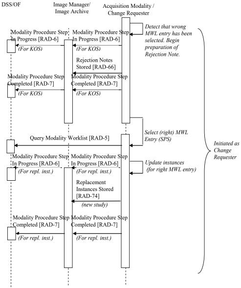
Figure 28.4.4-2: Acquired Images are Relevant to Correct Procedure
