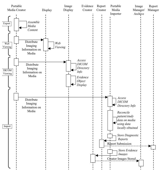
Figure 15.3.2-1: Portable Data for Imaging Process Flow
