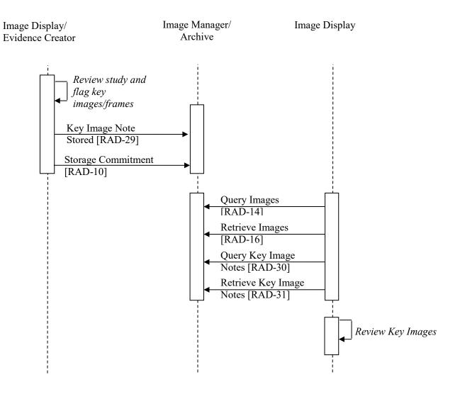
Figure 37.4.2.4.2-1: Process Flow in Key Images in DBT Screening Use Case
