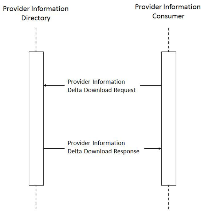
Figure 9: Provider Information Delta Download (CH:PIDD) interaction diagram
