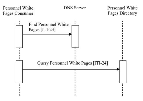
Figure 11.3-1: Basic Process Flow in PWP Profile
