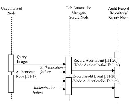
Figure 9.4.2.2-1: Unauthorized Node Process Flow
